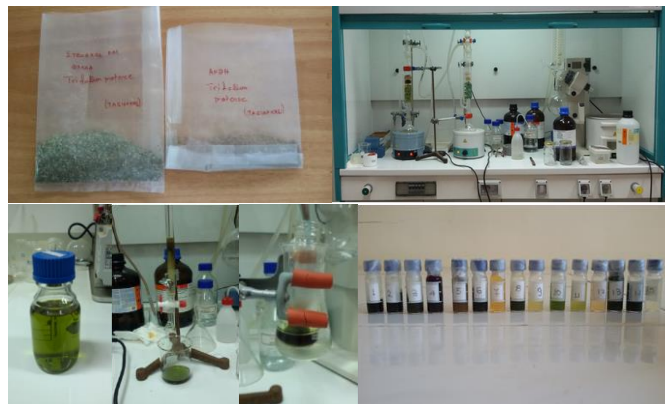
Figure 4. T. pratense samples after grinded in the mill and stages of extraction.
